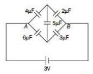
5. In a network, four capacitors C1,C,,C3 and C4 are connected as shown in the figure.
